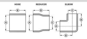
Silicone Class "A", 4 Ply Polyester Reinforced -55°C to +175°C [-67°F to +347°F] Conforms to SAE J20 (20R1 HD SW)
